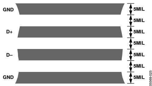
Figure 35. Typical Arrangement of Signal Tracks
